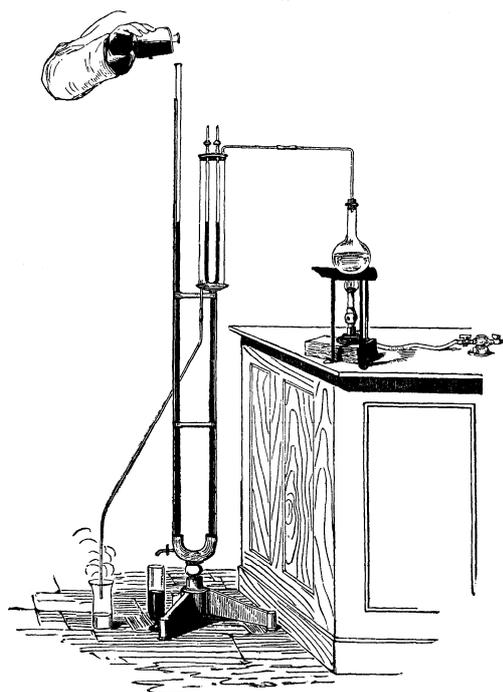
Figure 10: Demonstrating the gas laws (from Hofmann 1862-6, p. 415).
